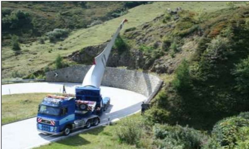
Plate 4-5 Blade adaptor transport system
