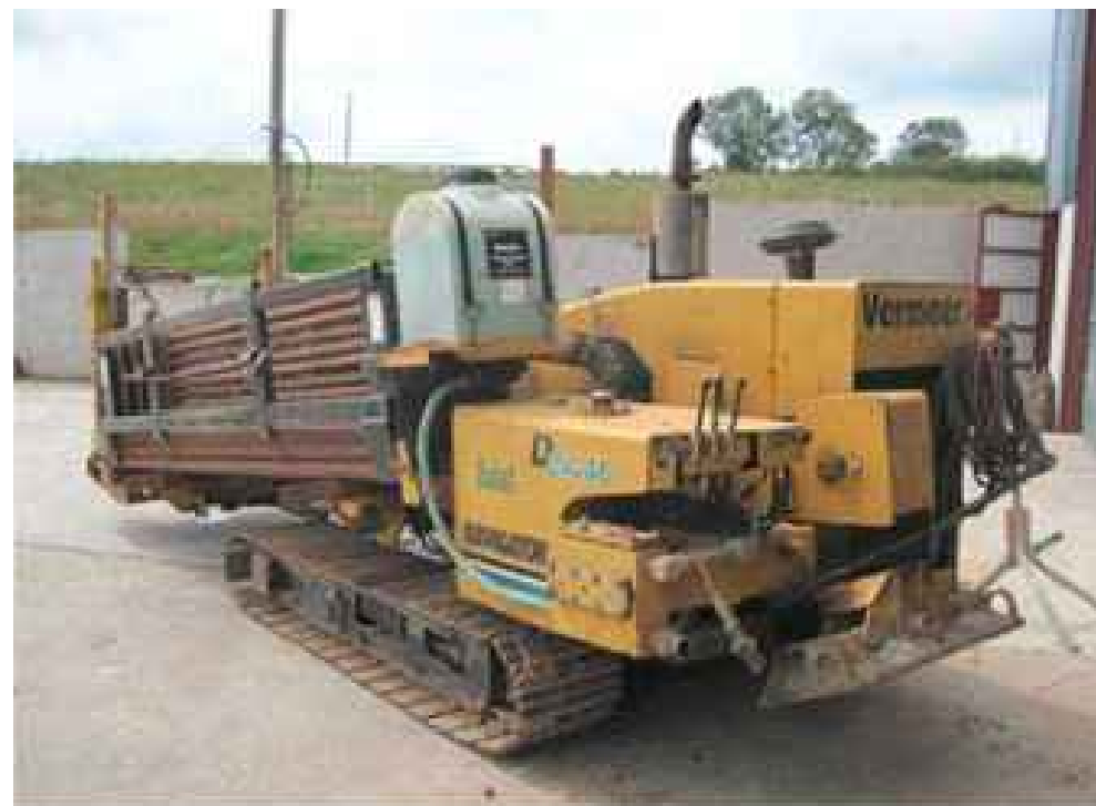
Directional Drilling Rig
