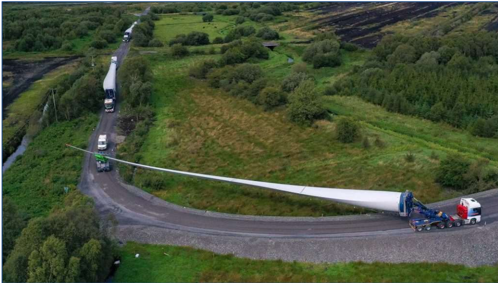
Plate 4-4 Clamp and Dolly system
